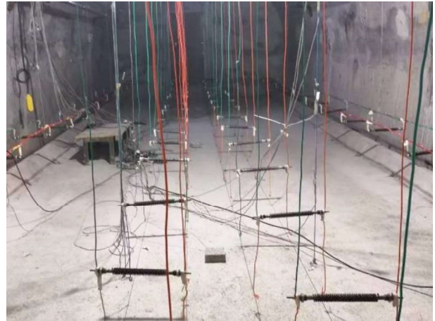
(b)The layout of heating tubes
