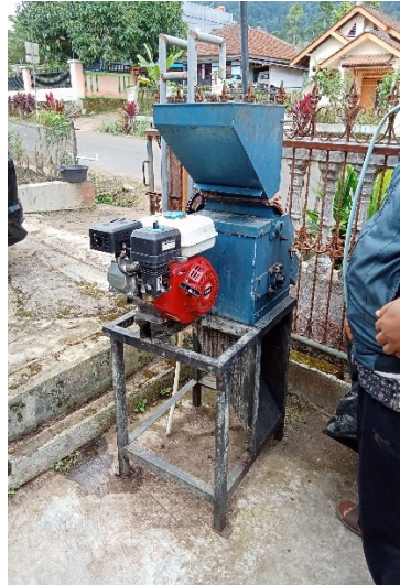
Figure 14. A pulper purchased with government support in Tribudisyukur, West Lampung. Belonging to an OFG producing mixed Robusta, certified and non-certified.
