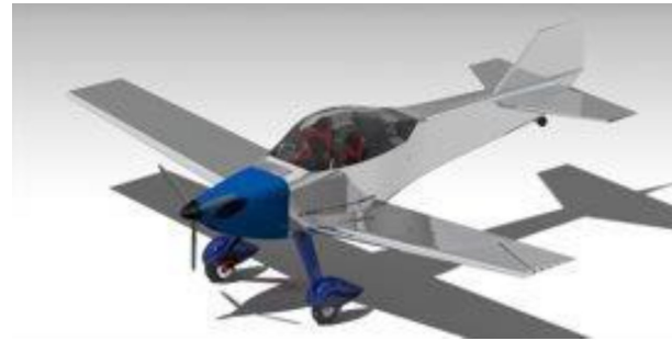
Figure 5. Example design from the capstone aircraft design module: A two-seat sport electric aircraft.
