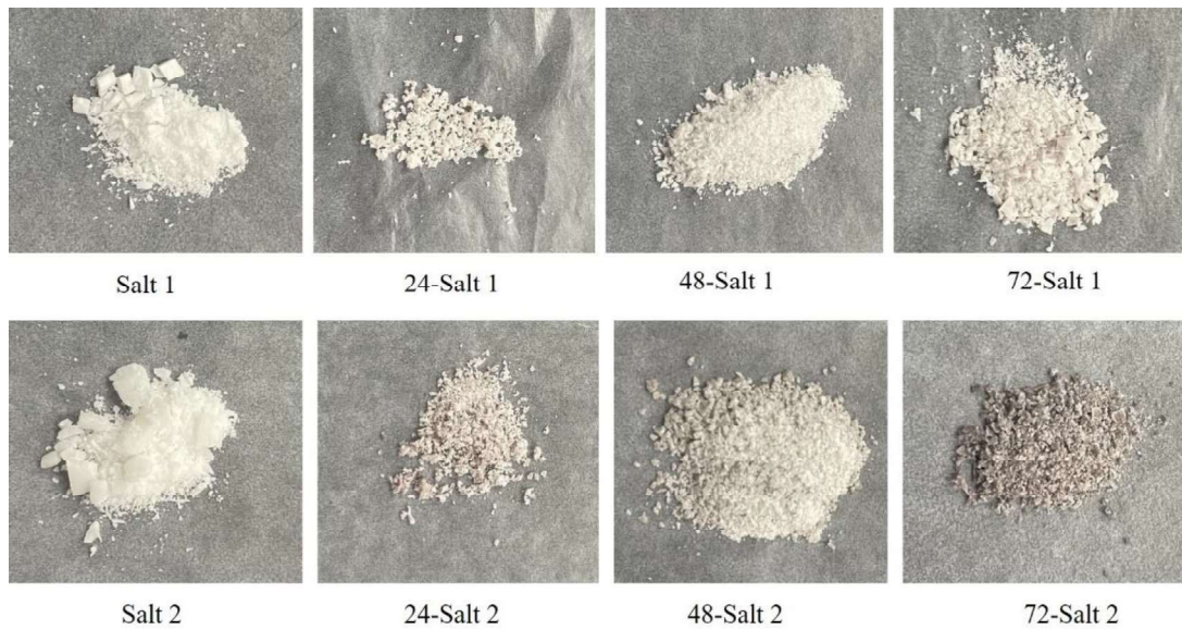
Fig.7. Macro-morphologies of ternary chloride salts before and after corrosion conducted at 650 °C for different time.
