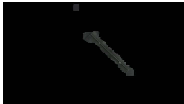
Figure 5. Region of interest over the weld seam line with each of the patches.
