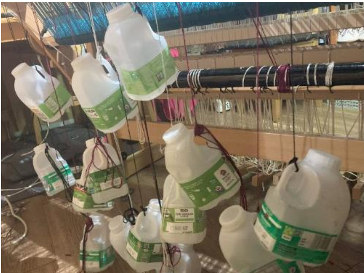
Figure 126 Nicola Moody, Loop, in progress, weighted milk bottles applying different amounts of tension to yarn, 2024
