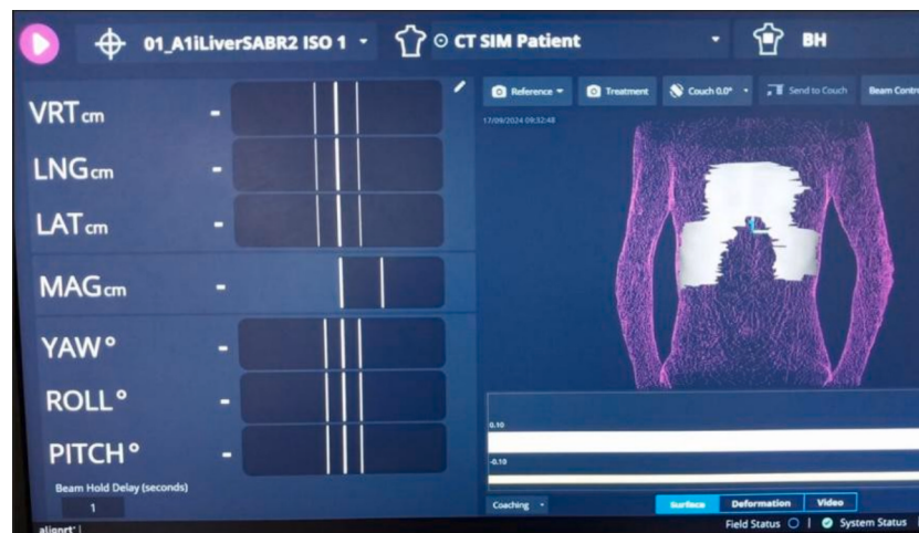
Fig. 2. SGRT surface capture with patient specific region of interest in white 1. Patient surface capture (purple) 2. Patient specific ROI (White) 3. Patient positioning deltas in 6 degrees of freedom (Vrt, Lng, Lat, Yaw, Roll, Pitch) 4. Patient breath amplitude gauge 5. Patient Plan identification 6. Treatment tools.
