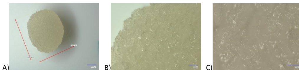
Figure 2.1: Micrographs of chitosan microspheres formed using salicylic acid taken on Keyence digital microscope. A) x30 magnification with measurement bars. B) x150 magnification C) x400 magnification
