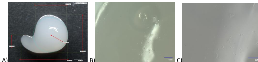
Figure 2.2: Micrographs of chitosan microspheres formed using acetic acid taken on Keyence digital microscope. A) x30 magnification with measurement bars. B) x150 magnification C) x400 magnification
