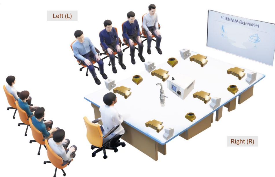
Fig. 1. Meeting-room layout showing participant seating and the approximate placement of ESP, C-PAS, Sterivex/SKC, OPC and APS instruments around the table.
