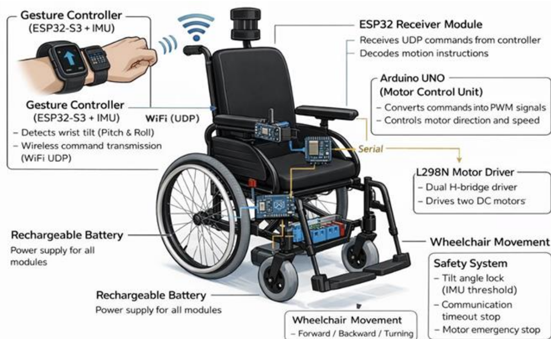
Fig. 1. System architecture of the gesture-controlled smart wheelchair.
