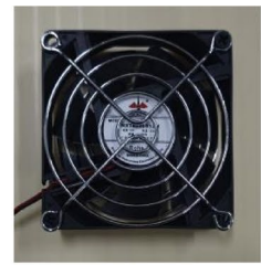
(c) Server cooling fan
