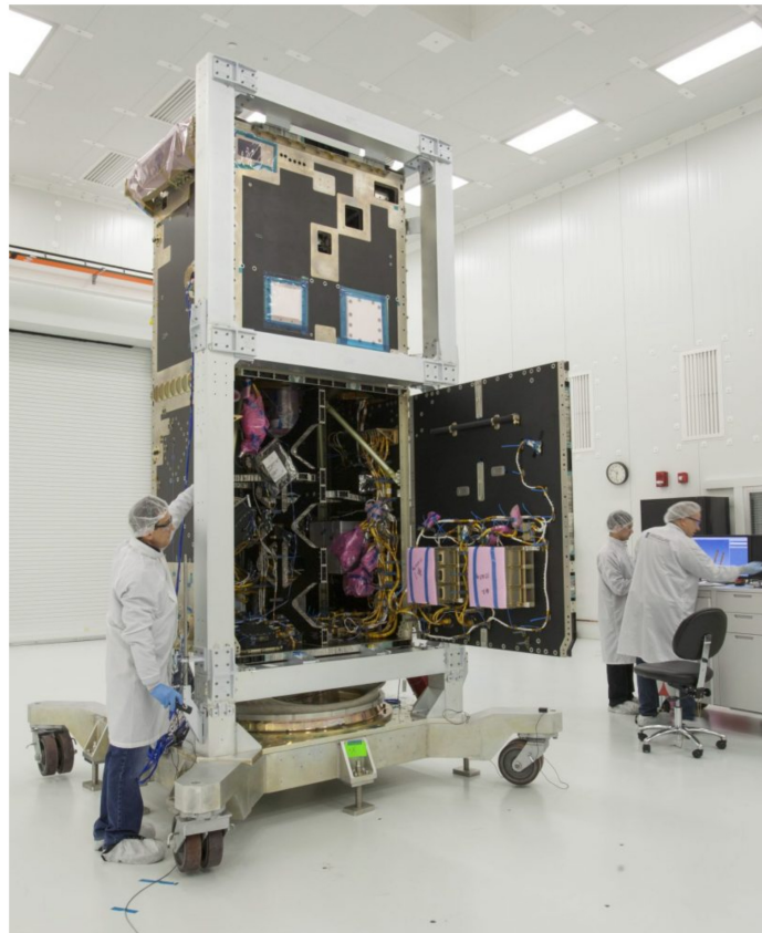
Fig. 7 CASTOR will be mounted on the MAC-200 satellite bus from Magellan Aerospace Corporation. This bus is pictured during the assembly of the Radarsat Constellation Mission which launched in 2019. For more details, see Sec. 2.5.
