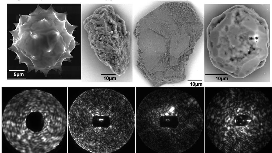
**Figure 2.** SEM images (top) and scattering patterns (bottom) of, from left: *Matricaria recutita* pollen, rough and smooth mineral dust grains and rough ice analogue plate.
