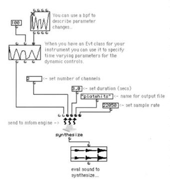
Figure 6. Breakpoint function control of a simple struck plate instrument.
