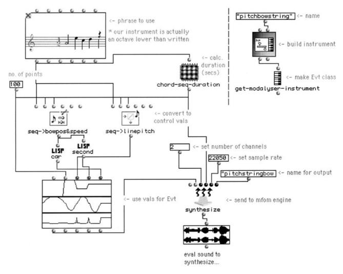
Figure 10. Control of a bowed string with variable pitch using standard notation.
