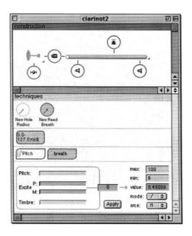
Figure 1. A Modalys-ER reed instrument with construction at the top, techniques at the bottom.
