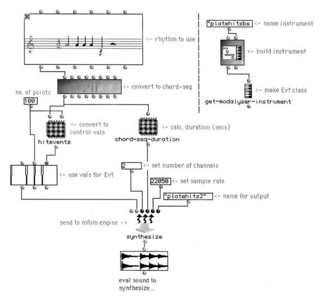
Figure 7. Control of a simple struck plate instrument with standard notation.
