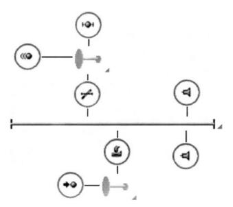
Figure 9. A bowed string instrument, using the top mass as the bow and the bottom mass as a finger with a fingerboard connection for pitching the string.
