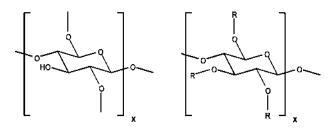
R= -CH<sub>3</sub> of -CH<sub>2</sub>CH(CH<sub>3</sub>)OH of -H
