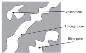
Figure 2: Different pore configurations<sup>[73]</sup>
