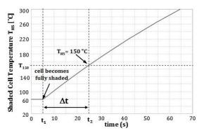
Fig. 5. Temperature trend over time in the fully shaded cell, for the operating conditions reported in [23].
