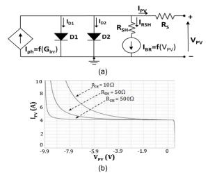
Fig. 1. (a) Considered electrical model for PV cells. (b)  $I_{pv}$  as a function of  $V_{pv}$  for three different values of  $R_{sh}$ , with  $G_{irr}$ =500W/m<sup>2</sup> and  $I_{ph}$ =4A.
