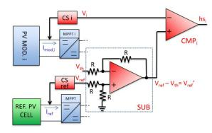
Fig. 10. Proposed implementation of the hysteresis comparators in HCMPi.
