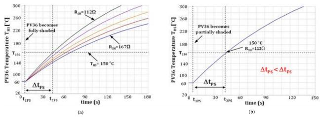
Fig. 7. Results obtained with our model for the behavior of the  $T_{HS}$  temperature of PV36 when: (a) PV36 becomes fully shaded after  $t_{1FS} = 5s$  ( $\gamma$ =0.01) and for various values of  $R_{SH}$ ; b) PV36 becomes partially shaded after  $t_{1PS} = 5s$  (with  $\gamma$ =0.3) and with the lowest value of  $R_{SH} = 112\Omega$  (worst case condition for the cell temperature).
