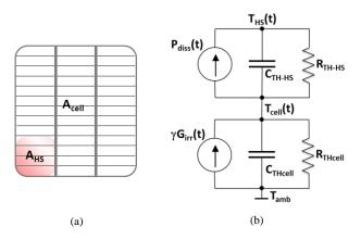
Fig. 4 (a) Partial shaded PV cell undergoing hot-spot condition; (b) Equivalent thermal model to estimate the time dependence of the temperature of the portion of the PV cell ( $A_{HS}$ ) under hot-spot condition.
