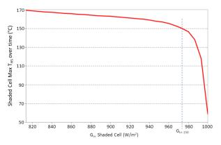
Fig. 11. Temperature increase in the cell area under hot-spot in a shaded cell, as a function of the cell irradiation density.
