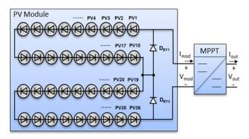
Fig. 2. Considered PV module architecture with distributed MPPT.
