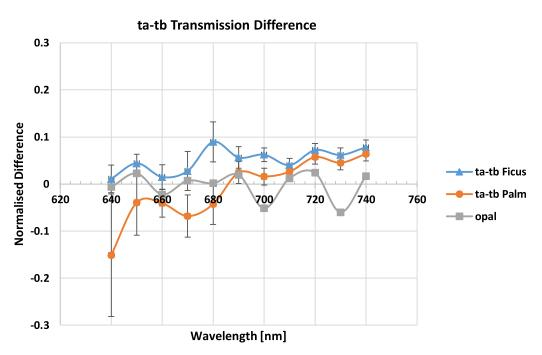
Fig. 6. Normalised transmission differences calculated from the data in Fig. 4. Error bars are  $\pm 3\sigma$ . The large excursions in the opal glass 'standard' are reproducable.
