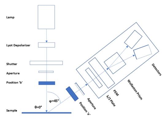
**Fig. 1.** Instrument diagram. The figure shows the scattering 'R' measurement configuration with the incidence angle  $\theta = 0^{\circ}$  and the observation angle  $\varphi = 45^{\circ}$ . Positions 'a' and 'b' are the locations of the narrow band filter discussed in the text.
