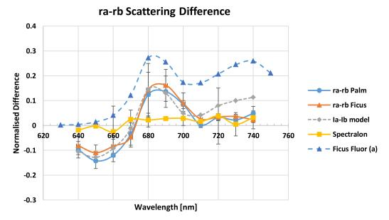
**Fig. 5.** Normalised scattering differences calculated from the data in Fig. 3 and including the Spectralon scattering standard. The error bars are  $\pm 3\sigma$ . Also included is an la-lb curve derived from the simple model in the Discussion section and a scaled plot of the fluorescence spectrum of *ficus* using a 405 nm laser diode in the 'a' configuration.
